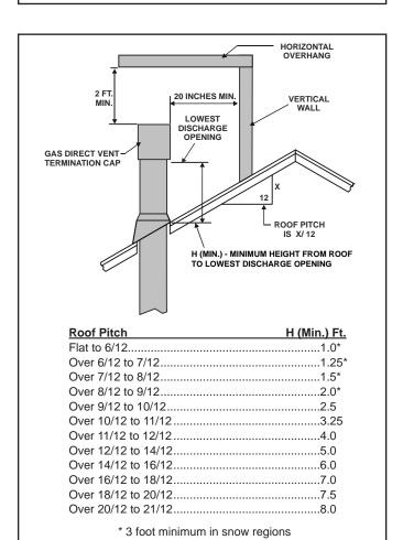
Figure 6.1 Minimum Height From Roof To Lowest Discharge Opening
